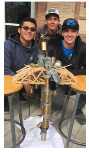
Kent Kast's physics class was tasked with designing mini-bridges from wooden popsicle sticks. Using the laws of physics to determine potential strength and durability, the student creations were tested for structural integrity by piling on weights up to the point of collapse. The winning bridge, designed by Jordi, Caleb, and Nathaniel, held up all the weights available—about 150 pounds!
